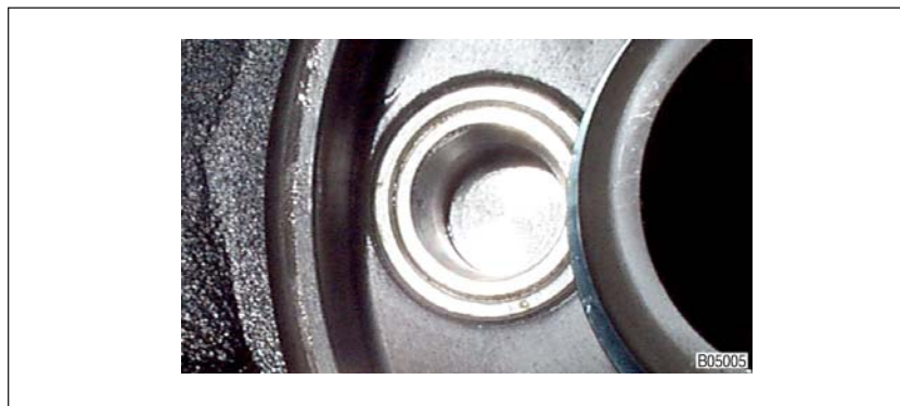
Figure 3. Bypass Valve Seated in Filter Base
